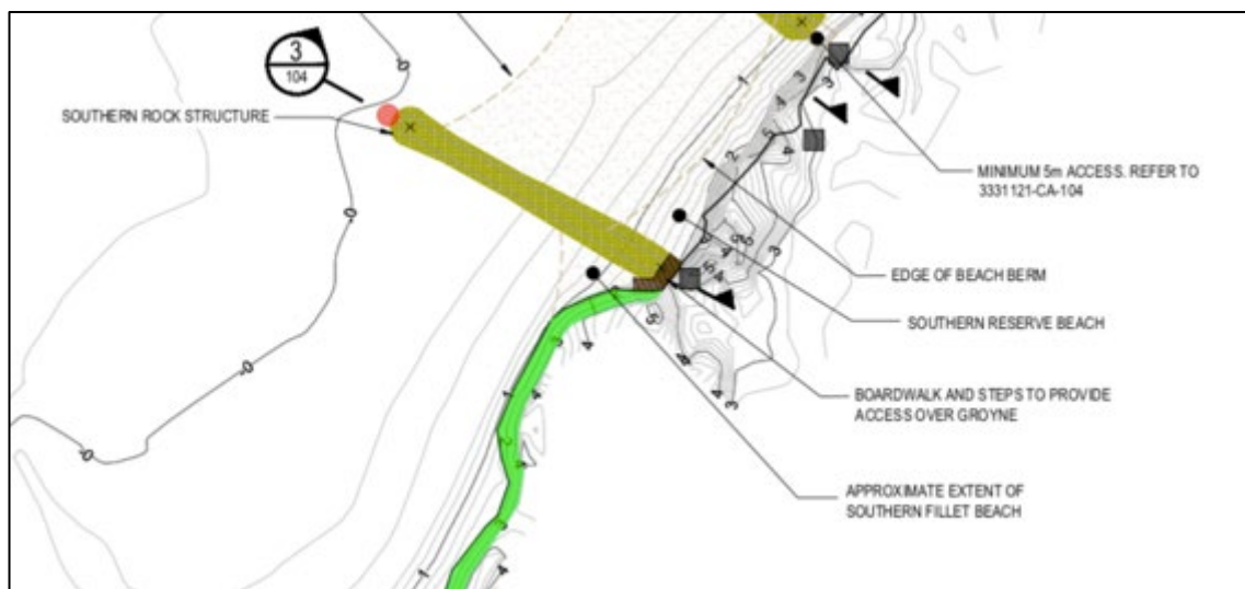
Figure 4: Extract from a design drawing showing the boardwalk (Source: Application)
