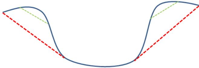
Figure 1: Cross section a typical waterway (blue solid line). Green dashed line is an example of 'battering'. Red dashed line is an example of 'bank or channel reshaping'.
