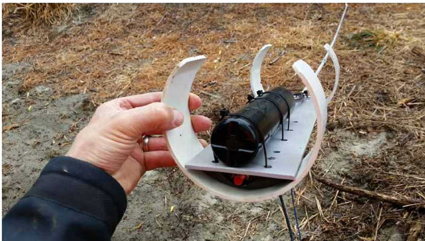
A dissolved oxygen sensor in its purpose-built cradle.
