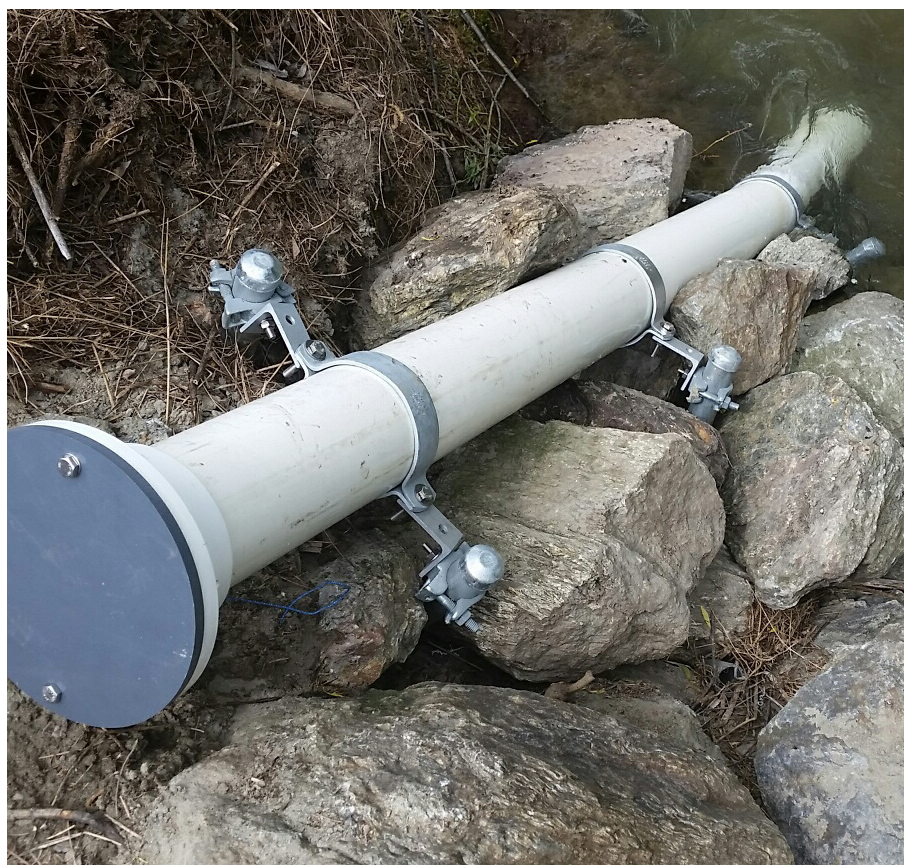
An installed dissolved oxygen sensor in the Cardrona River.
