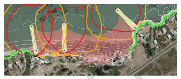
Mock-up of possible pre-determined visual monitoring zones for each groyne during construction. All areas outside of the amber areas are classified as green zone. Note: pre-determined visual monitoring zones will be finalised in conjunction with suitably qualified marine mammal expert prior to finalisation to EMP
