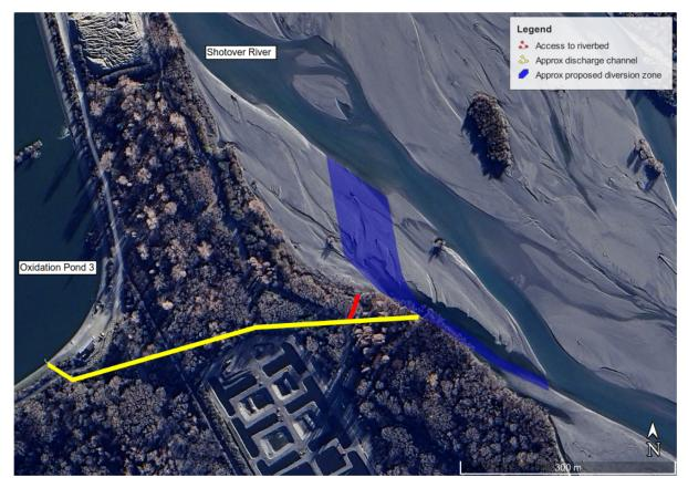
Figure 2: Discharge channel, proposed riverbed access and indicative proposed diversion channel works area. Note: imagery date is June 2024, with riverbed changes observed since then. (Source: Google Earth)
