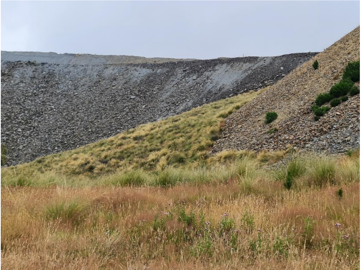
Figure 4. Photo of large aggregate deposited as 'screes' on the margin of the Coronation haul road.
