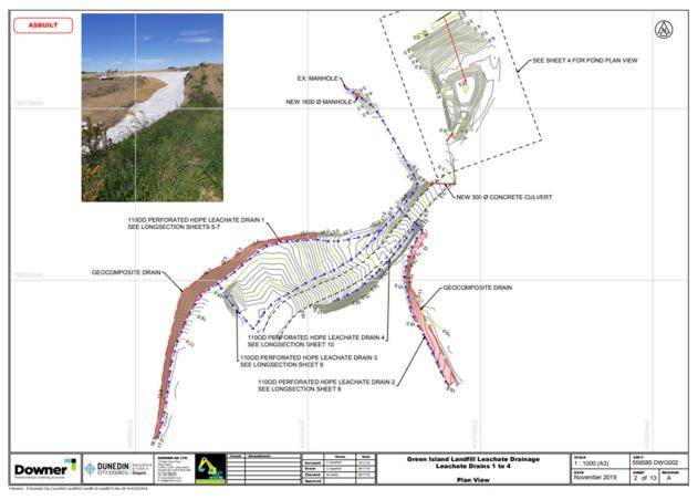
Figure 4 Northern leachate drains and pond
