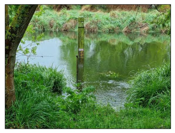
Photograph 16: Staff gauge 5 indicating the high water level.
