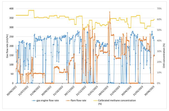
Figure 9 Methane concentrations, gas engine and flare flow rates 2021 - 2022
