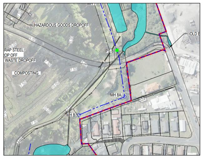
Figure 5 SE Constructed Wetland Culvert and Leachate Interception Trench Alignment (snip from Drawing C204)
