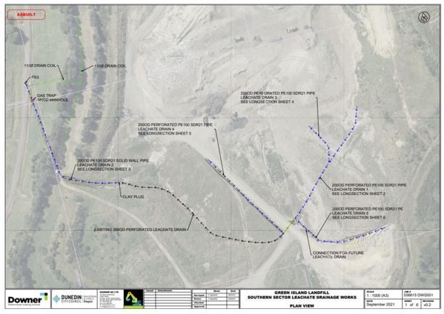
Figure 3 Asbuilt for horizontal leachate collection drain and connection to PS3
