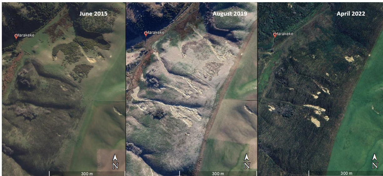
Figure 23. Time series photos of changes in vegetation cover and resulting erosion at the Harakeke monitoring site following aerial spraying in 2017 in preparation for planting of commercial forestry.
