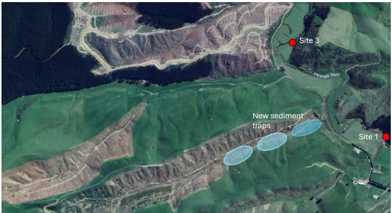
Figure 31. The sub-catchment area with recent commercial forest harvest and area of active erosion on adjacent farmland (including indicative locations of sediment traps) established in 2023 from which discharge into Te Hikapupu/Pleasant River was monitored with Aquawatch waka. Site 3 is upstream of the erosion-prone sub-catchments and site 1 is downstream of the sub-catchments.
