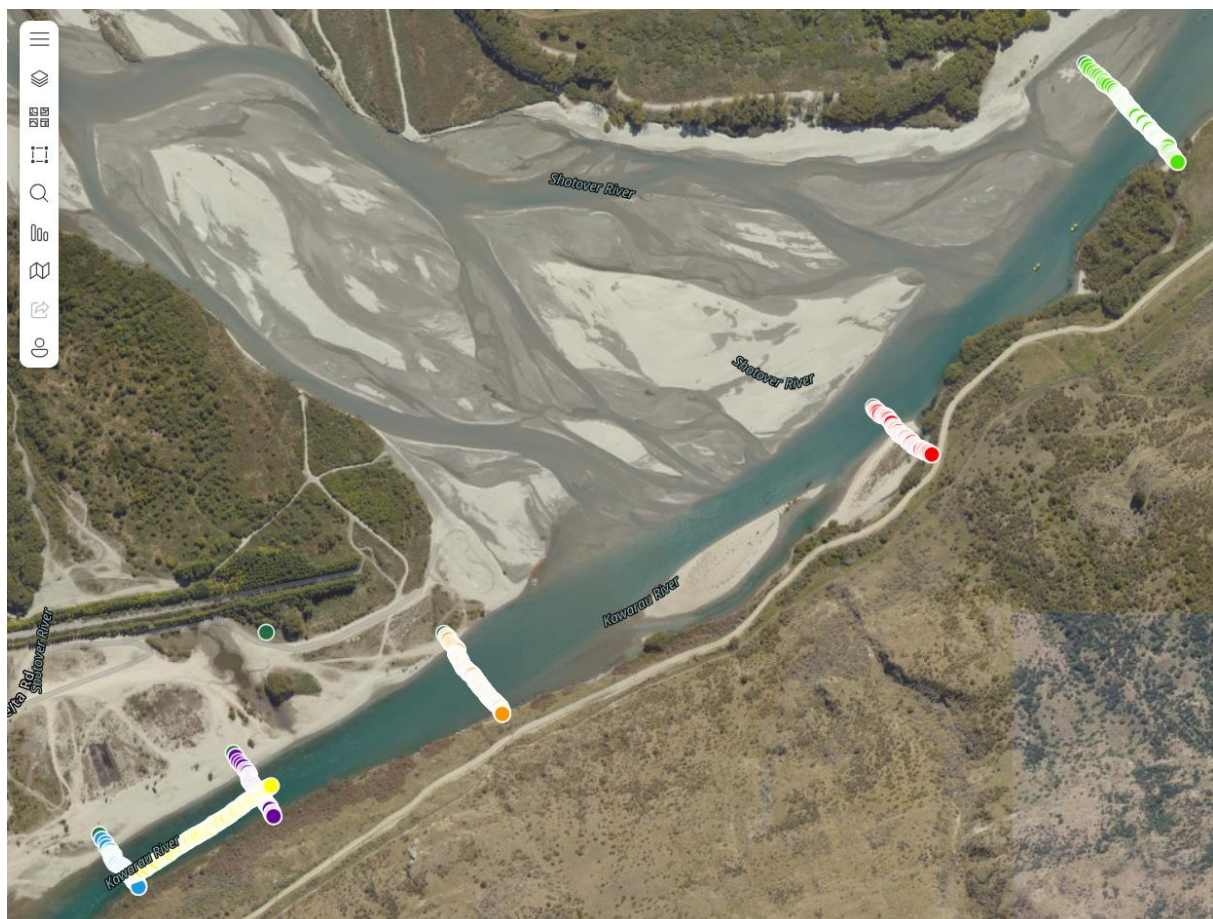
Figure 2-1: ArcGIS displaying ship-track transects of each cross-section.
