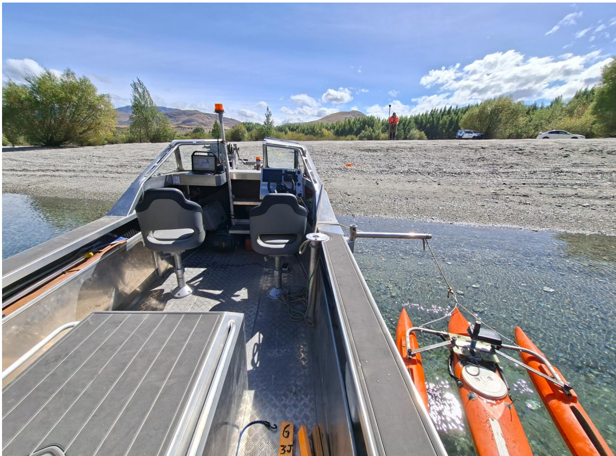
Figure 1-2: Jetboat with ADCP Riverpro profiler attached on sidearm, RTK-rover positioned at survey transect on bank.
