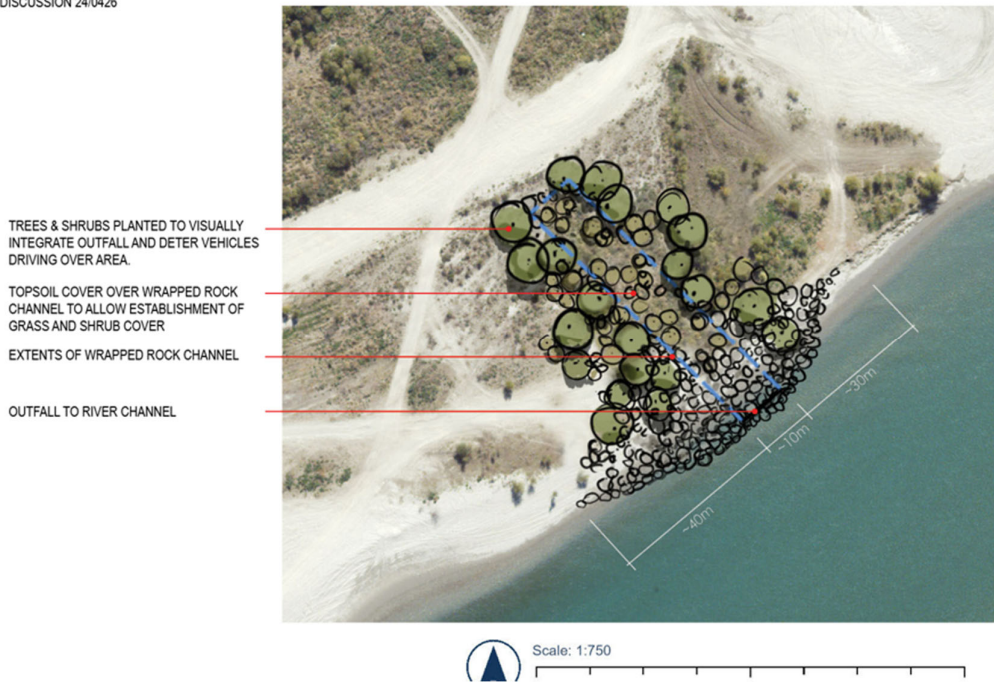
Figure 2.5 Rock outfall general arrangement drawing (indicative)
