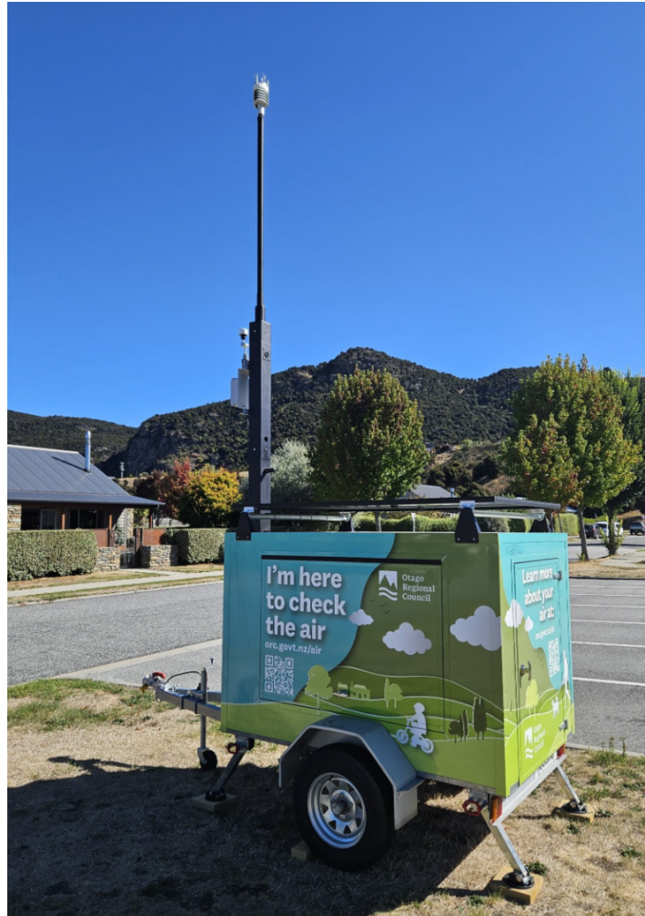
Figure 5: Mobile monitoring trailer in operation at Albert Town
