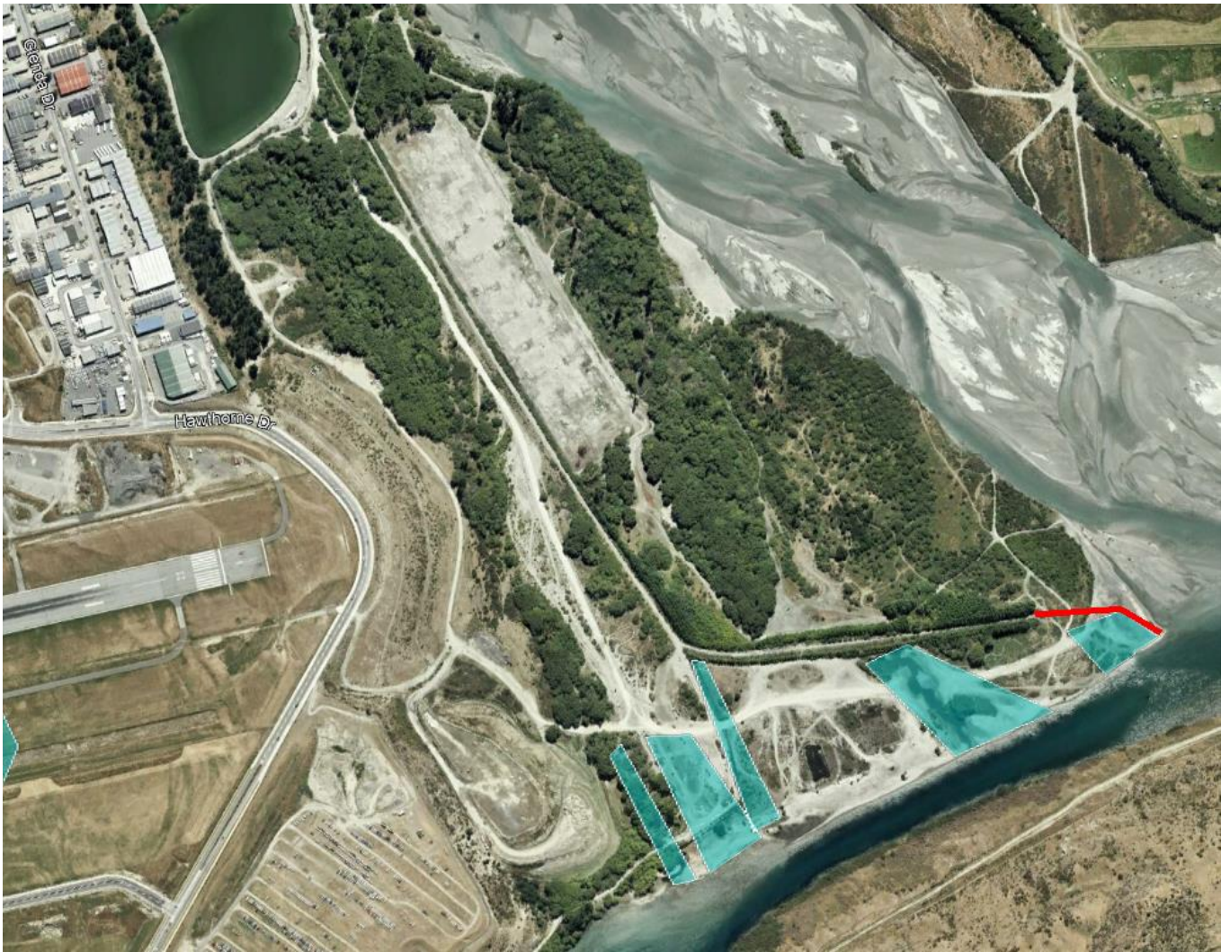
Figure 11 Option 4 b, figure indicates potential areas which could be used for engineered flow paths (blue highlight) and flood wall modification (red line)
