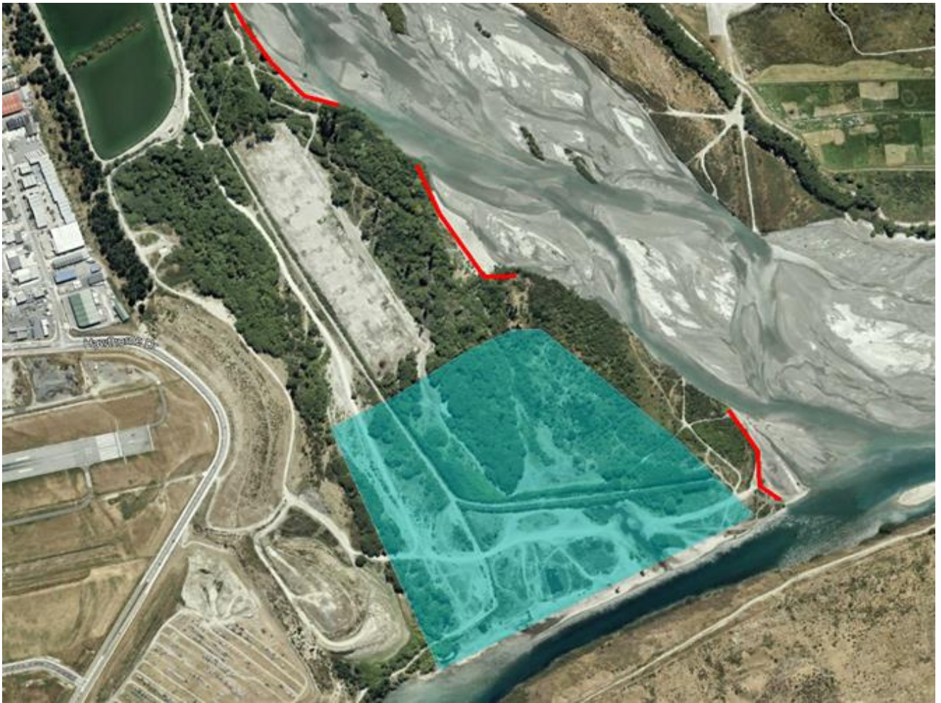
Figure 4 Option 1b Trenches in Shotover Delta, indicative site area (blue highlight) and flood wall relocation (red lines)
