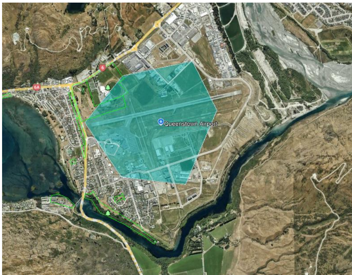
Figure 12 Option 5 a, possible injection wells at the Frankton flat area (blue highlight), not all highlighted land areas would be required, rather discreet points within the area
