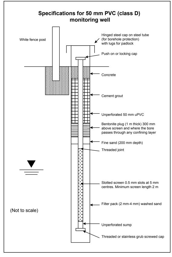
Figure 3.2 Details of monitoring well
