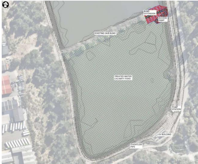
Figure 10 Expected area to be converted into a treated calamity pond (Beca, April 2022)
