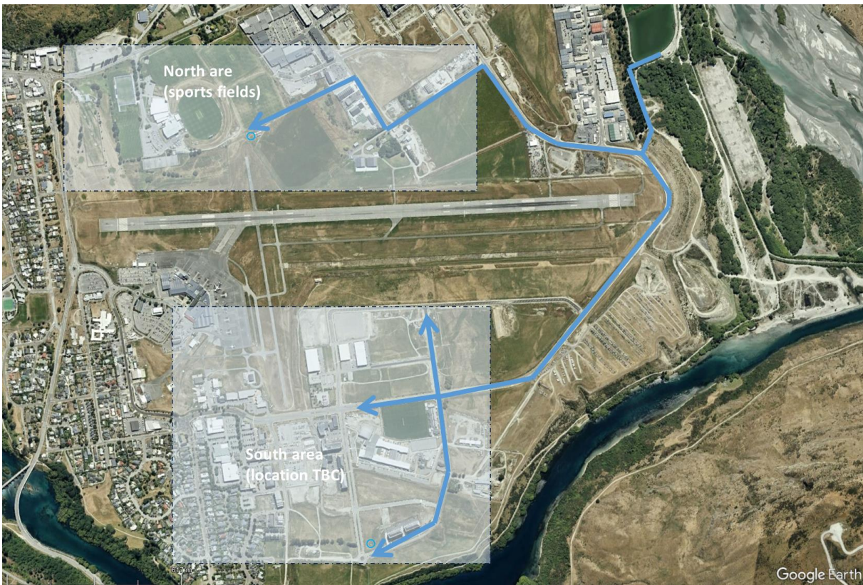
Figure 20 Indicative pipe routes (blue) from WWTW to Frankton Flats (exact locations to be confirmed)
