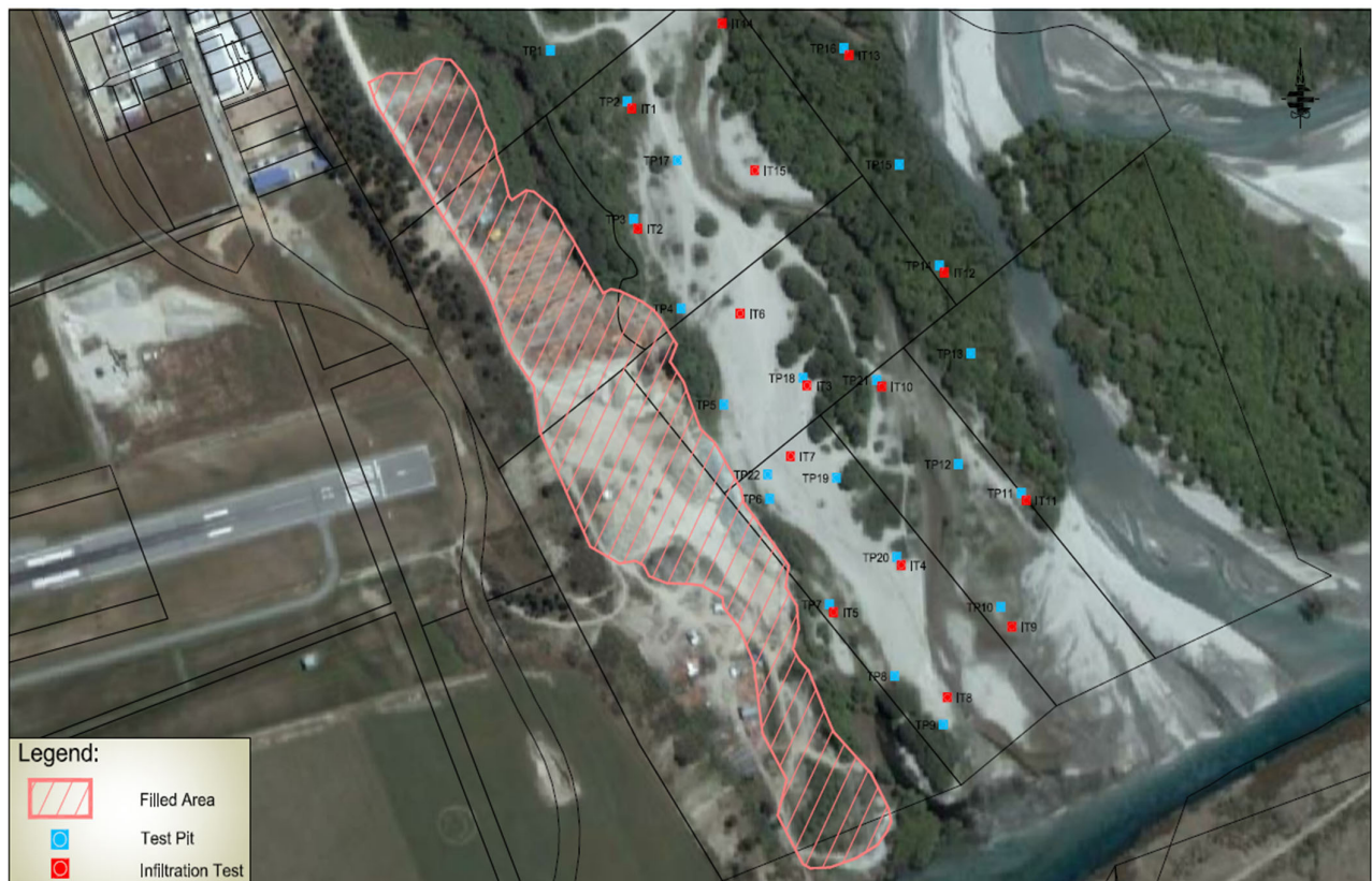
Figure 1 Shotover Delta Test Pit and Infiltration Test Location Plan (From Duffill Watts, 2008)
