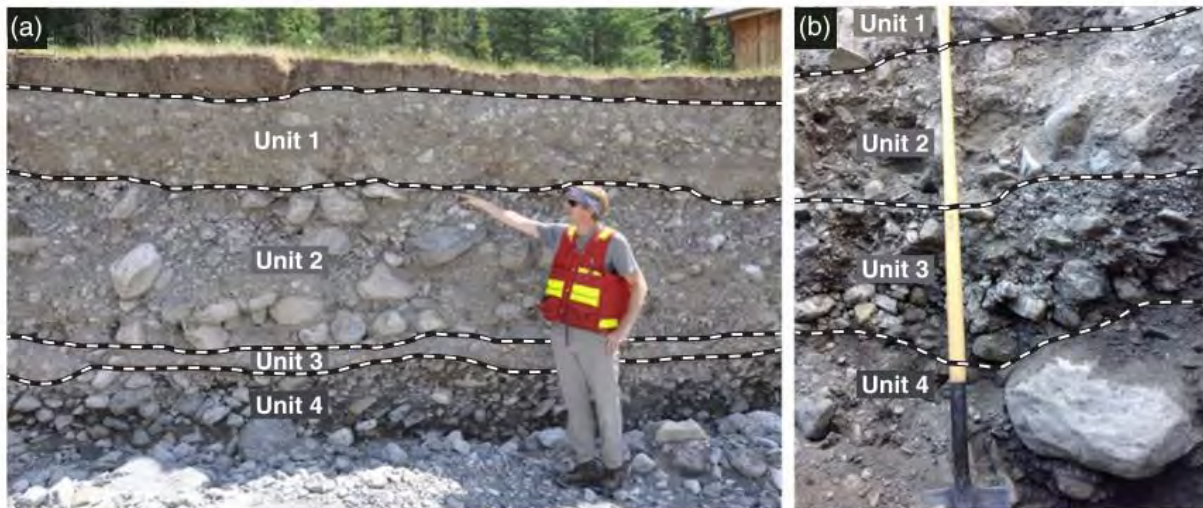
Figure 20: Typical debris flood stratigraphy from Cougar Creek, Alberta, Canada (Church & Jakob, 2020). Unit 1 is described as a matrix-supported outbreak flood deposit with little stone imbrication while Units 2 and 4 are high-energy debris flood deposits. Unit 3 is interpreted as a basal density flow (part of flow in contact with the ground) of Unit 2.
