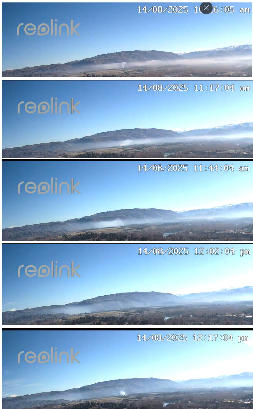
Figure 11: Camera images of smoke being emitted in Earnscleugh on the morning of 14th August showing a gradual collapse of an inversion
