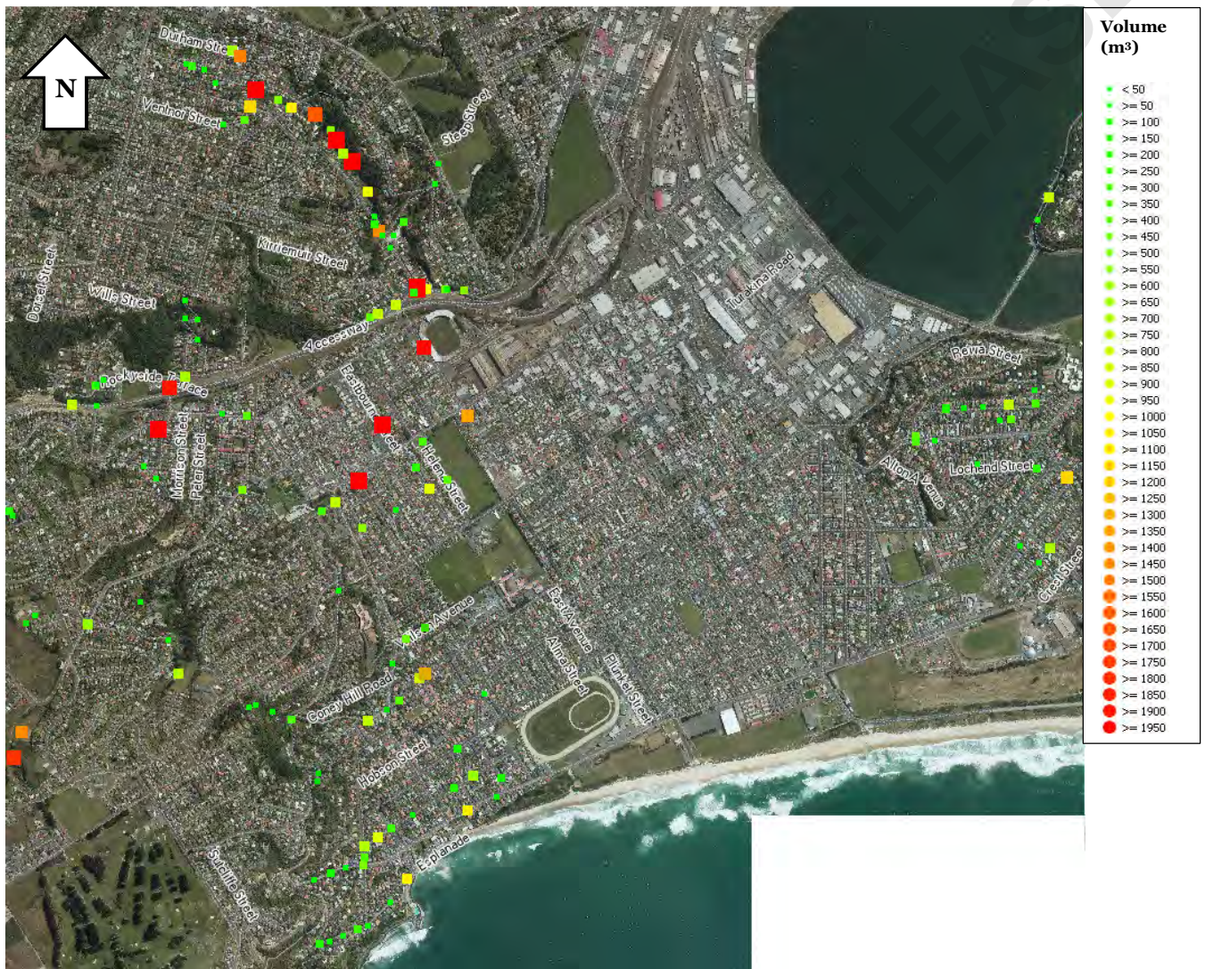
Figure 7 – Predicted wastewater manhole overflow volumes for the South Dunedin area (June 2015)
