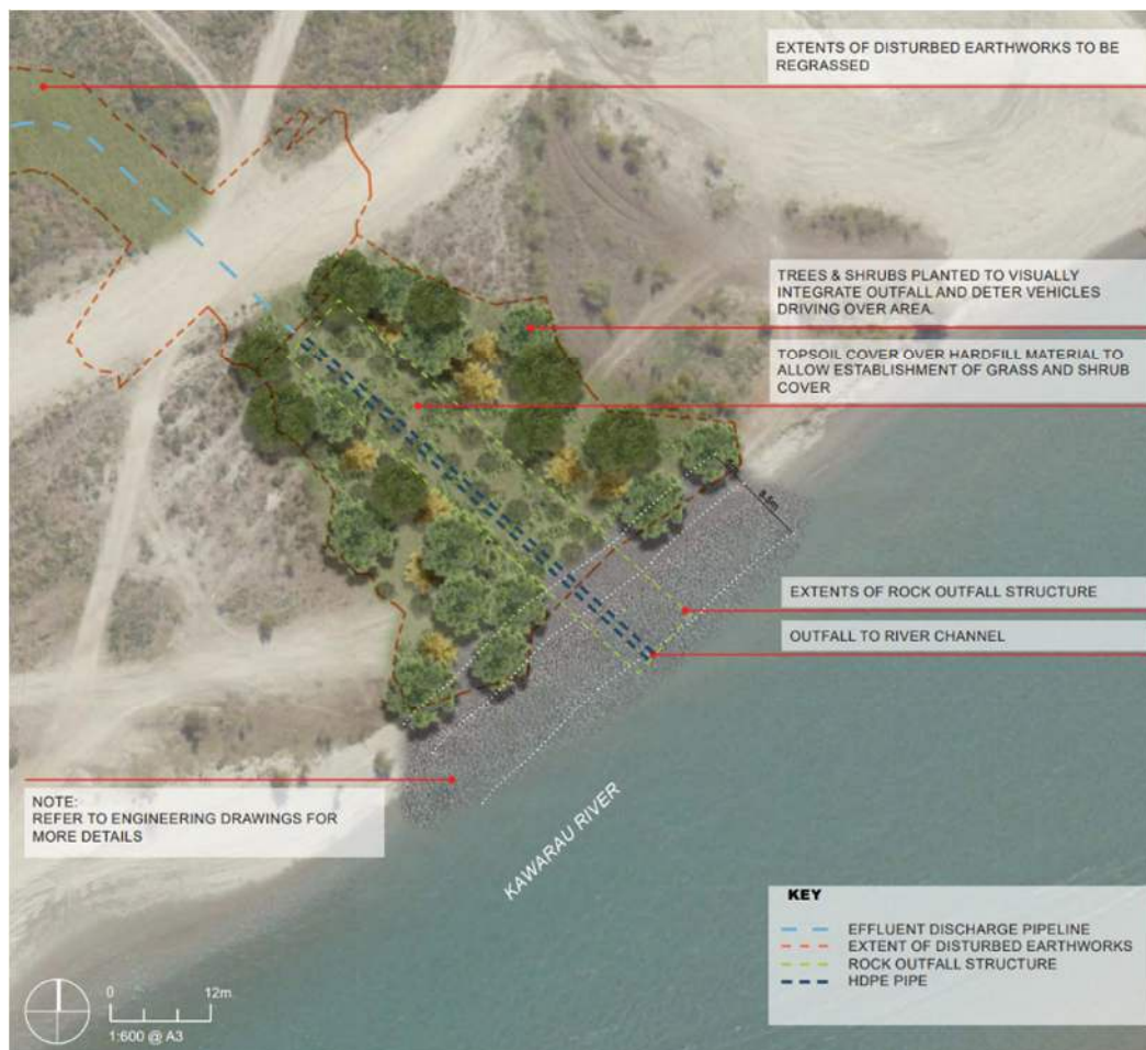
Figure 18: Indicative concept design for rock outfall (source: Boffa Miskell)
