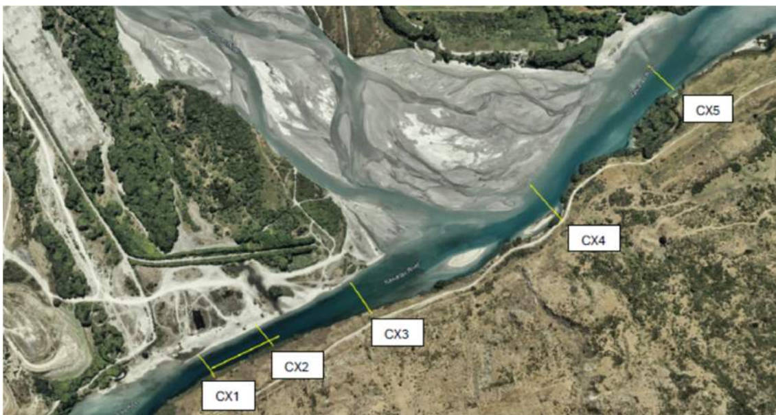
Figure 32: Kawarau River surveyed transect locations, as indicated by yellow lines with cross-sections numbered. Longitudinal profile indicated between cross-sections CX1 and CX2 (ESNZ, 2026)
