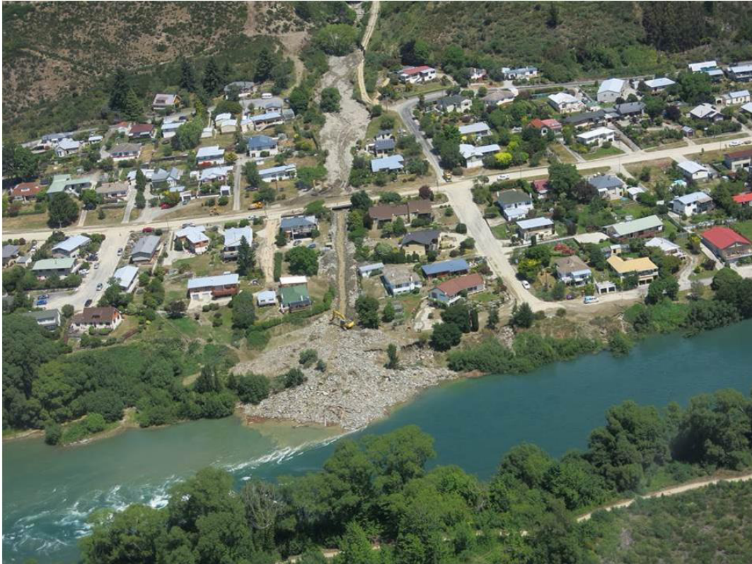
Figure 3. View up Reservoir Creek showing sediment and debris deposited at the confluence with the Clutha River – Photo taken by ORC staff on 27 November 2017. Excavator has cleared part of the channel in the middle of the view. Width of debris at river edge is approximately 70 m. The Clutha River flows from right to left.
