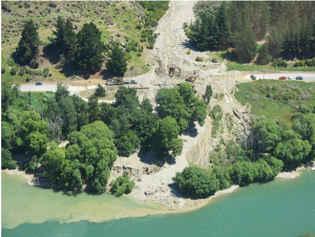
Figure 12. Sedimentation on the lower reach of Black Jacks Creek – 27 November 2017 (ORC staff photo). Width of view along the riverbank is 150 m.
