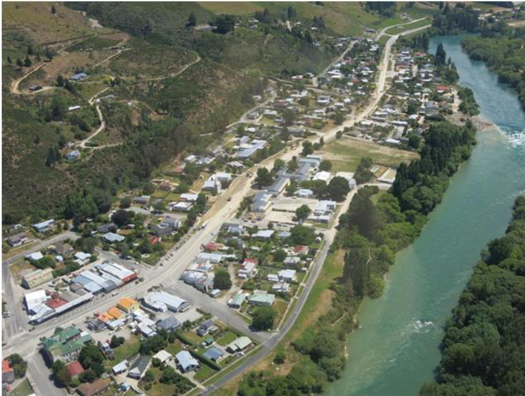
Figure 5. Sediment deposition in Roxburgh Township and in the Clutha River from Reservoir Creek – Photo taken by ORC staff on 27 November 2017. The sediment lobe from Reservoir Creek protruding into the Clutha River is visible in top right of image. Note the finer sediment deposited on SH8 in the centre of the image.
