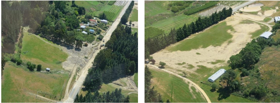
Figure 13. Sedimentation in the lower reaches of an unnamed creek, here referred to as Golf Course Creek– 27 November 2017 (ORC staff photos). In the left image, boulders inundated a paddock upstream of the highway. The right photo shows finer sediment (silt to small gravels) deposited across the rugby field.
