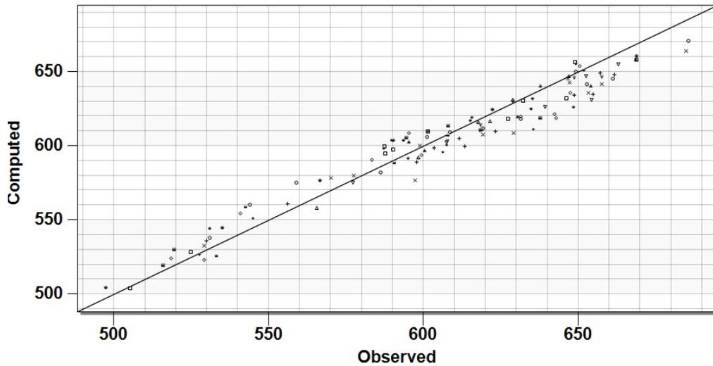
Figure 4.8 Steady state scatter plot (model computed vs observed head)
