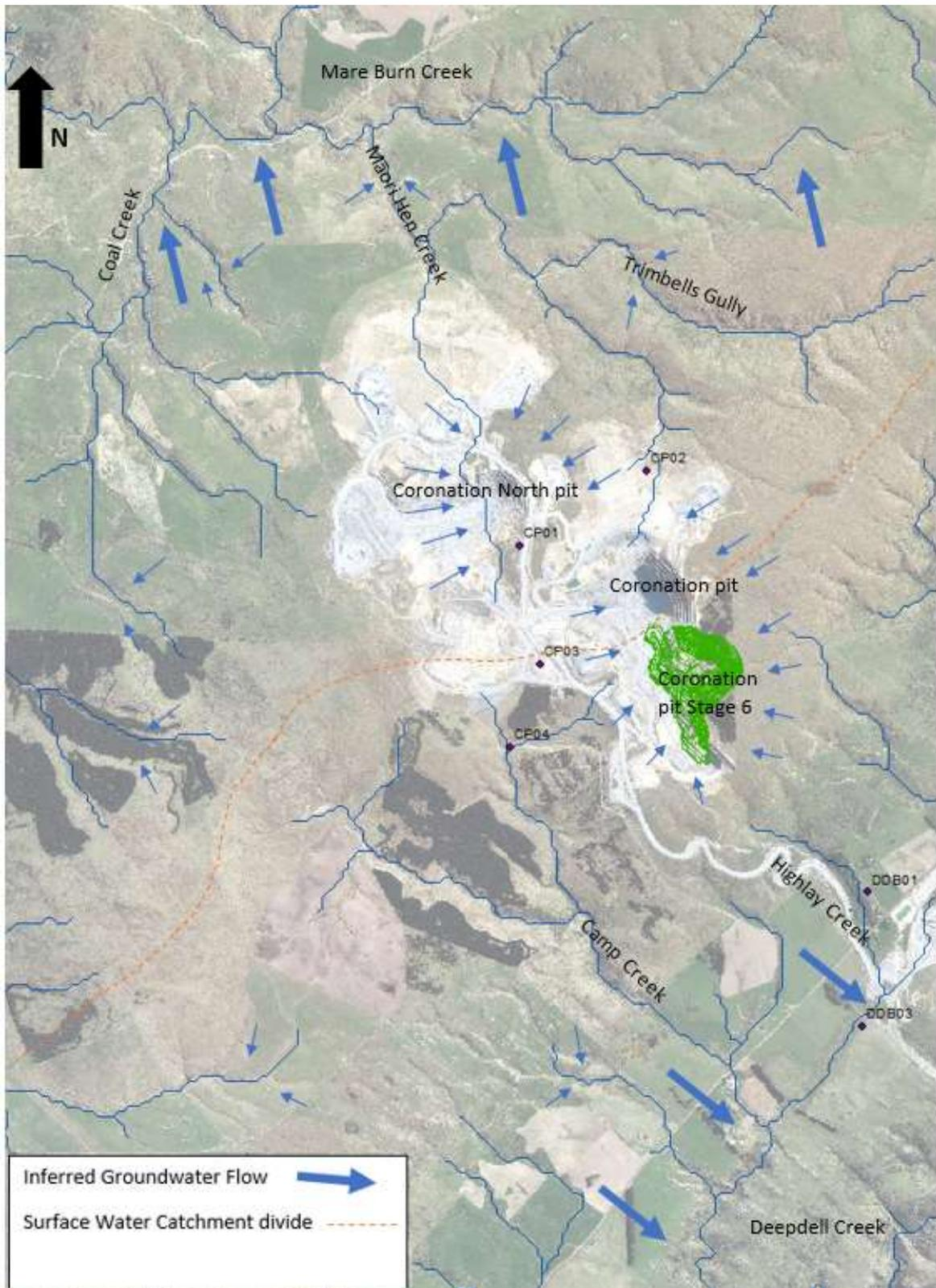
Figure 4.2 Inferred existing / proposed mining groundwater flow direction
