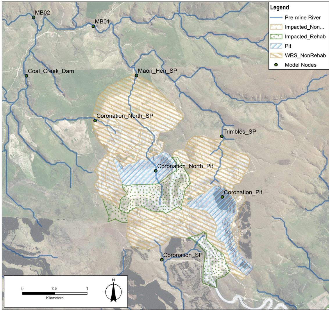
Figure 7.2 Coronation Waste Rock Stack Rehabilitated / Non-Rehabilitated Plan - Current
