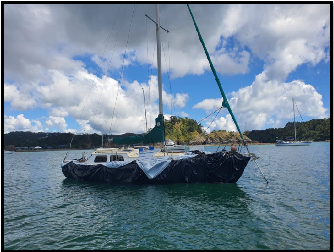
Figure 6: Example of encapsulation using a plastic sheet (Taronui Bay, Northland, 2022)
