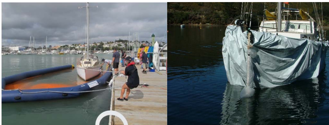
Figure 1. Examples of encapsulation using a floating dock and a plastic sheet (photo credits: Matt Smith, NIWA and Bruce Lines, Diving Services NZ Ltd).
