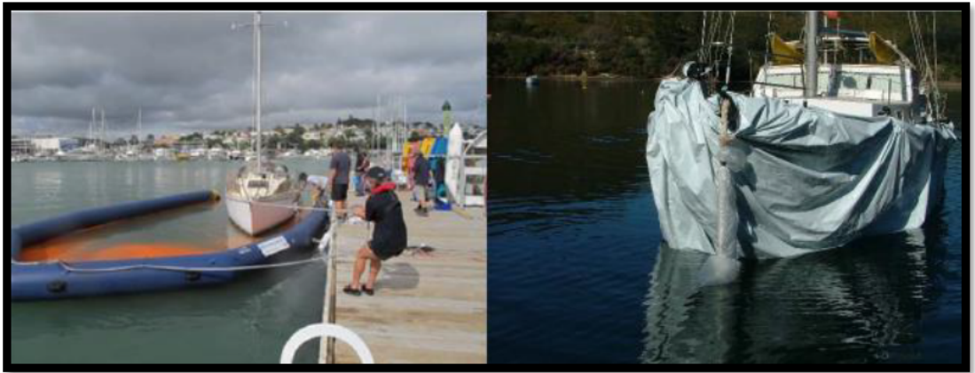
Figure 5: Examples of encapsulation using a floating dock and a plastic sheet (photo credits: Matt Smith, NIWA and Bruce Lines, Diving Services NZ Ltd).
