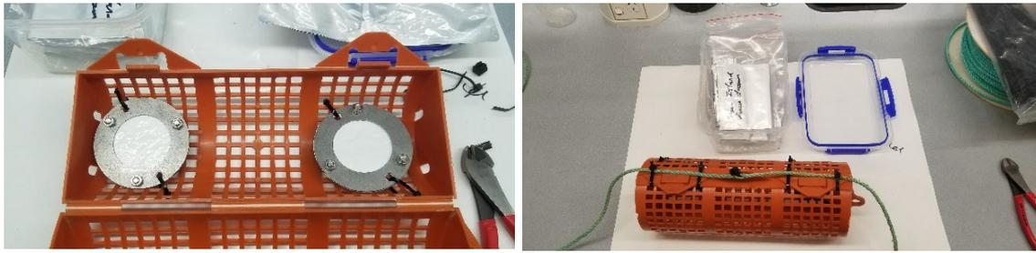
Figure 2. Preparation of surface water passive sampler devices.
