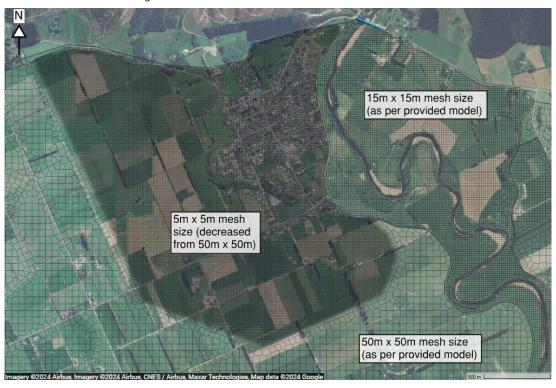
Figure 9-3. HEC-RAS model mesh resolutions within area of interest (Image source – Google Earth).
