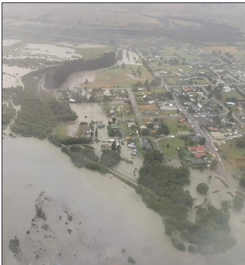
Figure 5.16 February 2020 – flooding of Glenorchy township residential area, due to high Rees River flows causing overtopping of a section of the Rees-Glenorchy floodbank.
