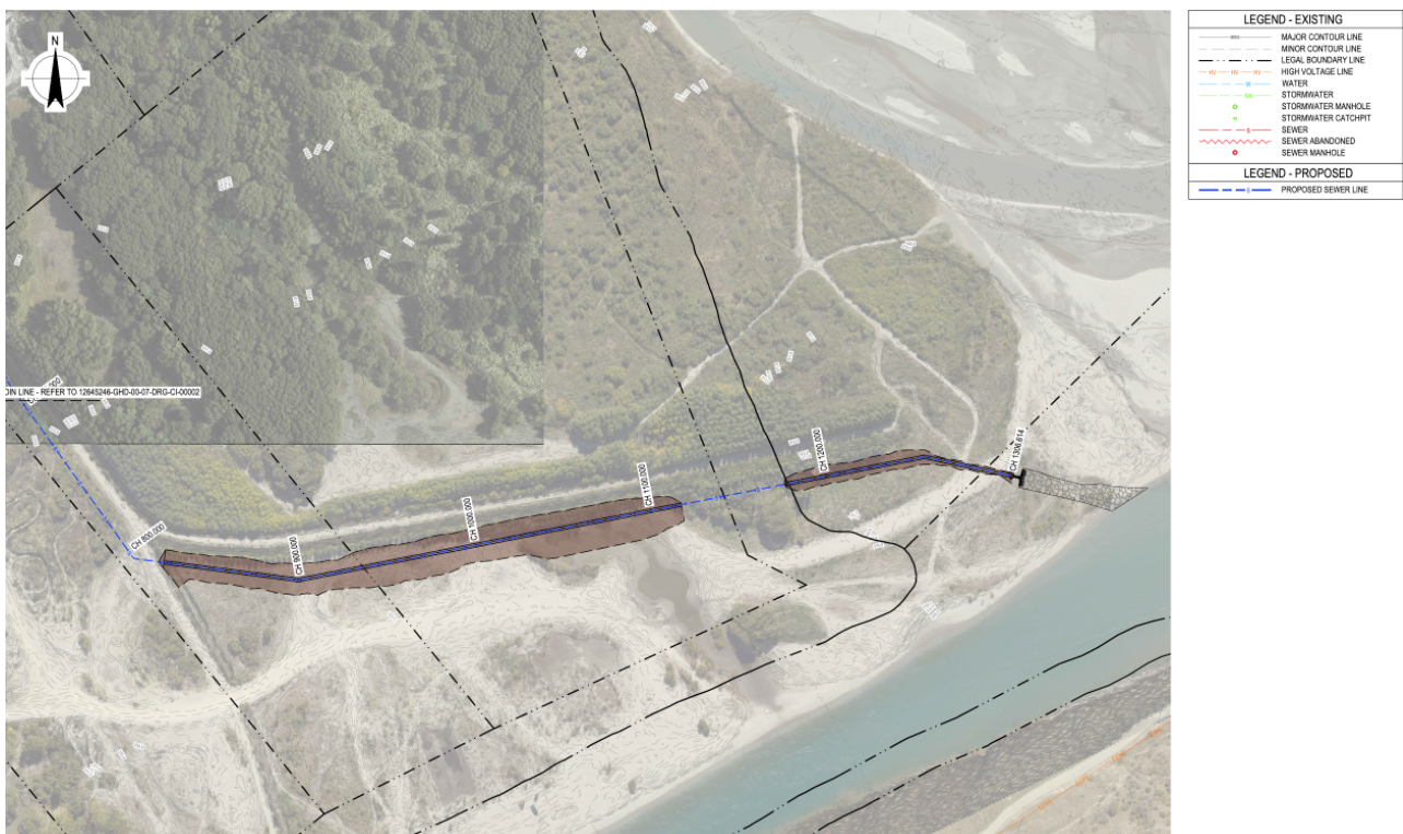
Figure 4: Current prelim design plan for pipe realignment and rock outfall into the Kawarau (supplied by GHD (2026))
