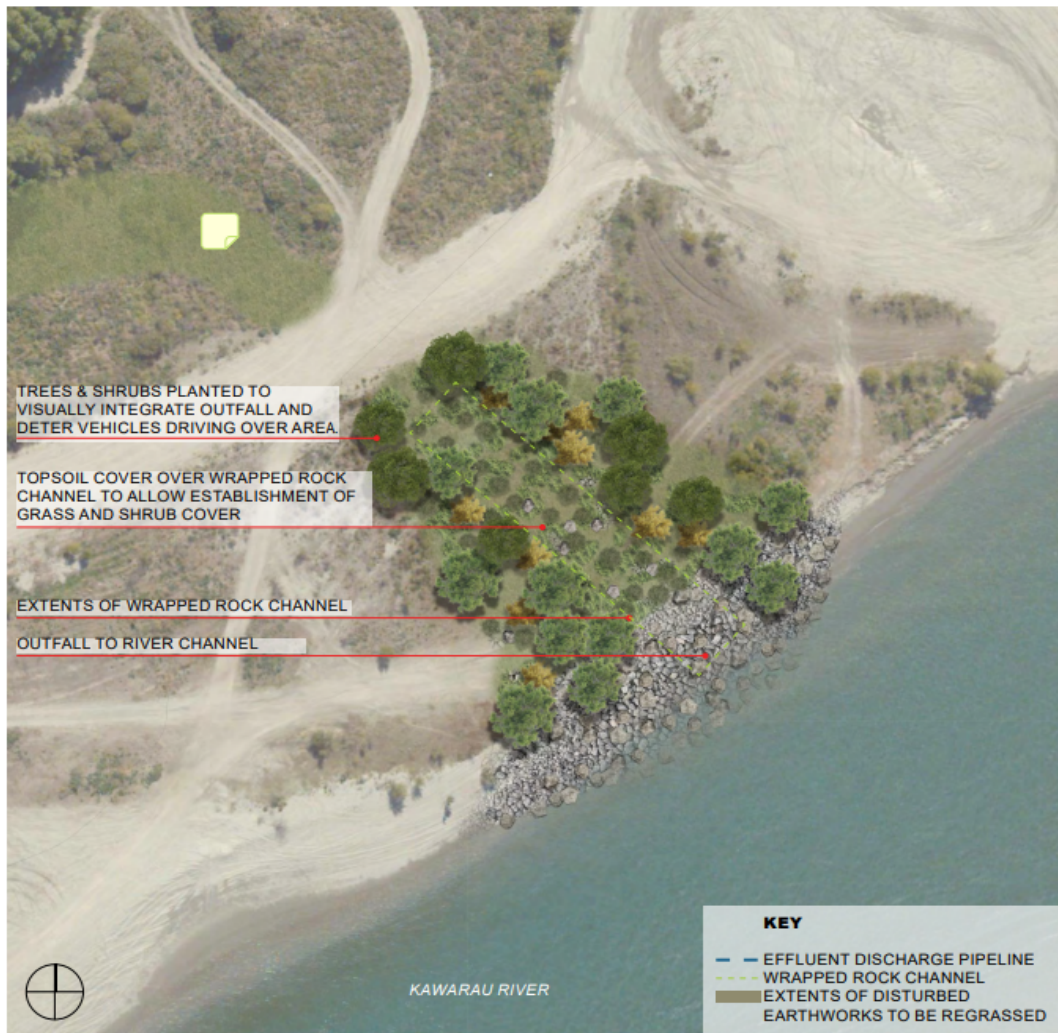
Figure 5: Preliminary rock outfall design and landscape mitigation planting (supplied by Boffa Miskell (2026))
