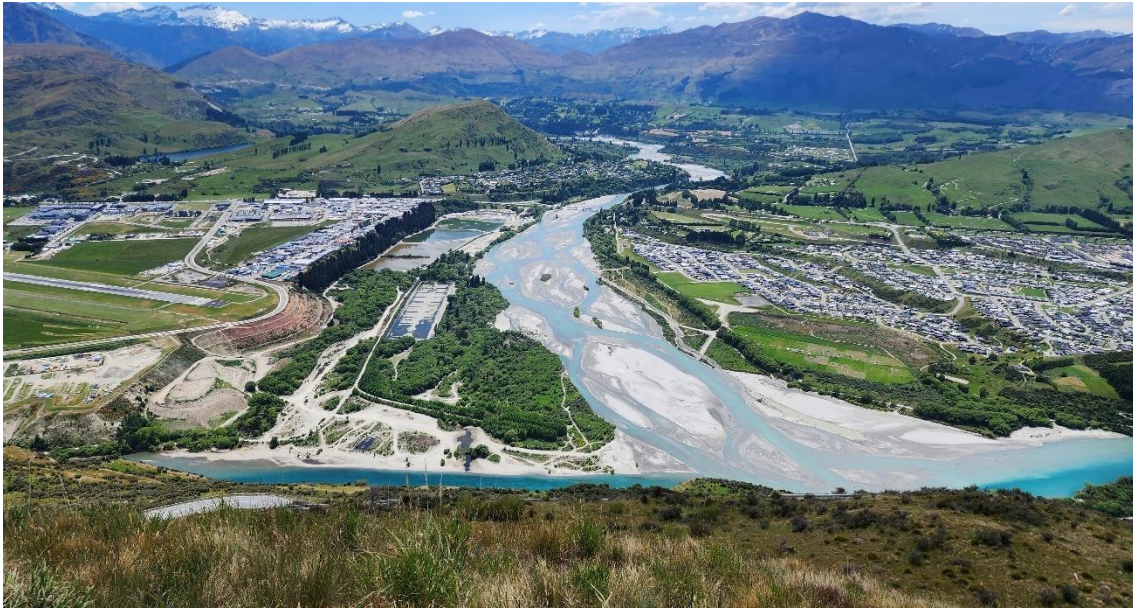
Figure 6: Kowarau River, and Shotover Delta, looking north from the Remarkables showing high suspended solids load in the Shotover River and on the left margin of the Kowarau River downstream of its confluence with the Shotover River. RS10 is located on the right side of the photo. Photo taken on 22 November 2023 with flows of 35 cumecs recorded in the Shotover River at Bowens Peak. Photo source: Dawn Palmer.
