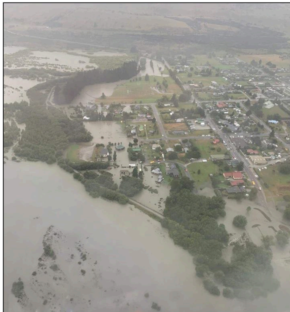
Figure 5.16 February 2020 – flooding of Glenorchy township residential area, due to high Rees River flows causing overtopping of a section of the Rees-Glenorchy floodbank.
