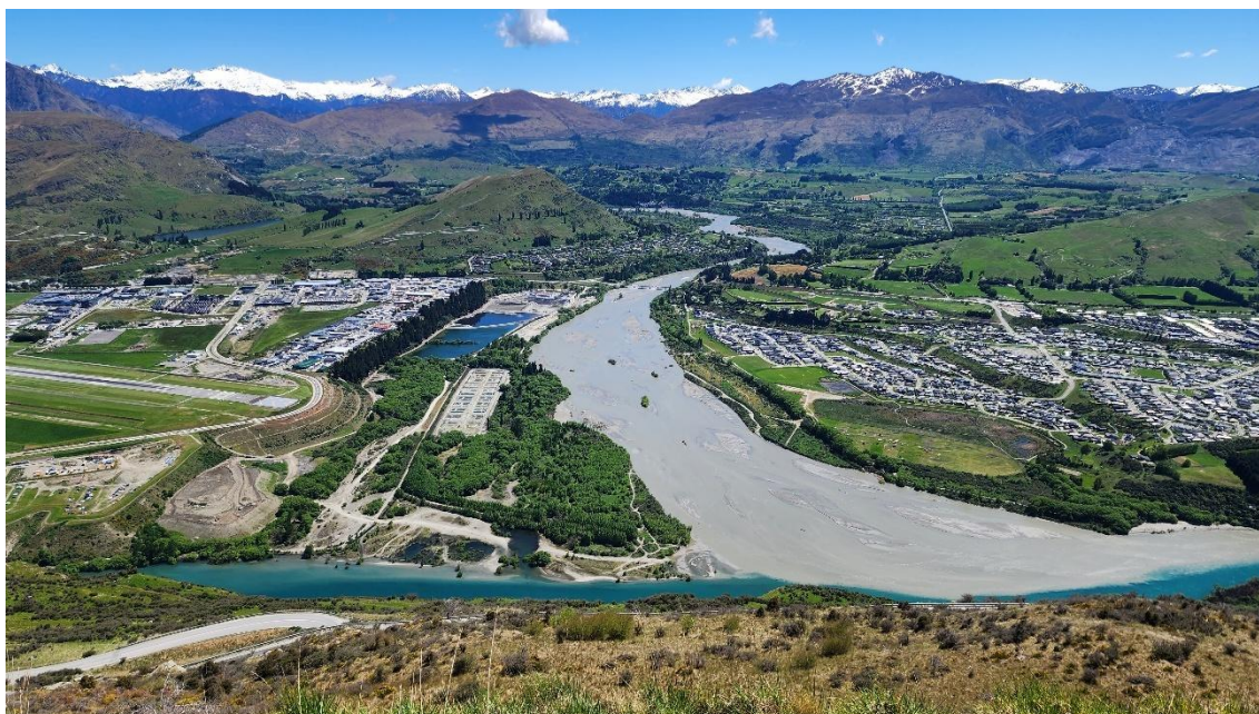
Figure 7: Kawarau River, and Shotover Delta, looking north from the Remarkables showing high suspended solids load in the Shotover compared to the Kawarau. Photo taken on 11 November 2025 with peak flows of 195 cumecs recorded in the Shotover at Bowens Peak. Photo source: Dawn Palmer.
