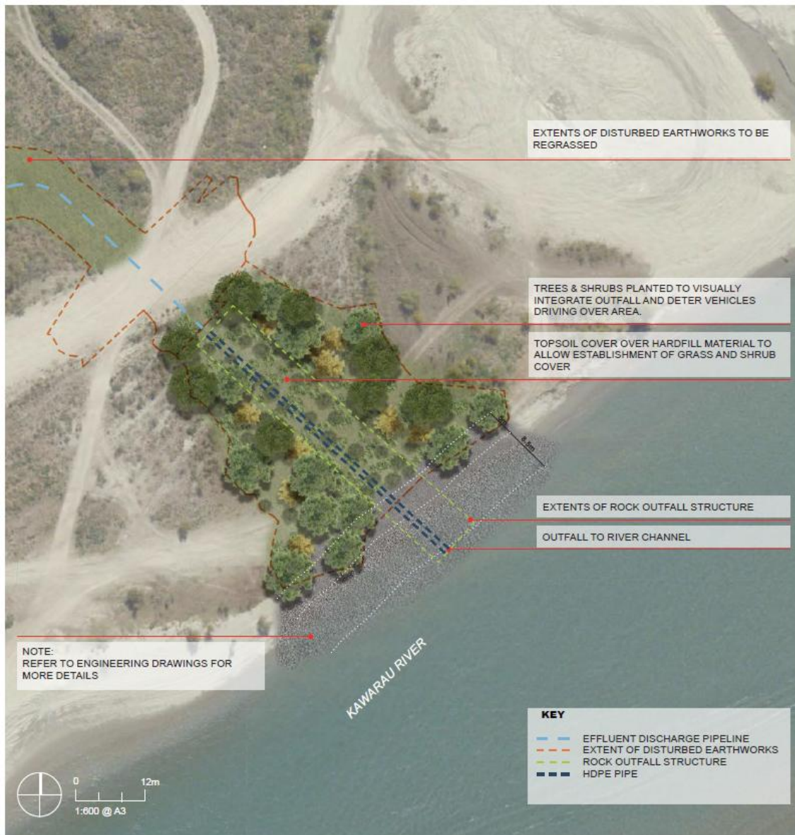
Figure 2: Proposed indicative design of outlet structure (to be confirmed in detailed design).
