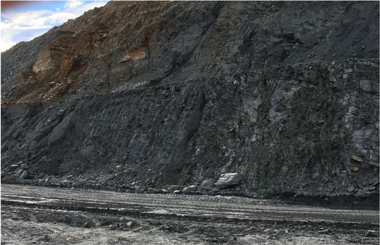
**Photo 4:** Coronation Pit Stage 2– eastern wall immediately south of the ‘fish bowl’. Westerly dipping faults can be seen outcropping at 270°.
