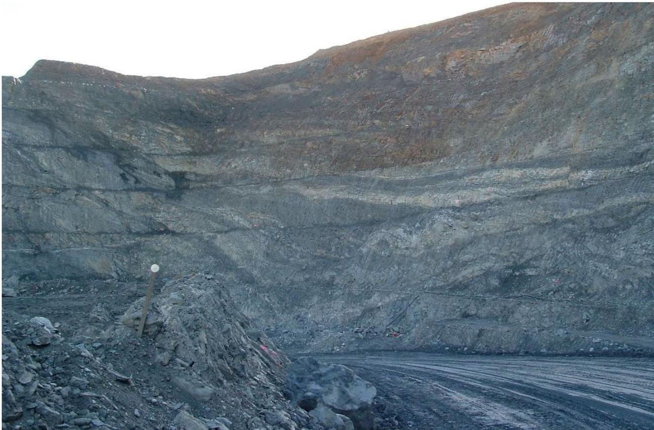
**Photo 7: View of north-east wall taken July 2005. Notice the depth of weathering, the prominent quartz veins, and the very good performance of the slopes in fresh rock.**
