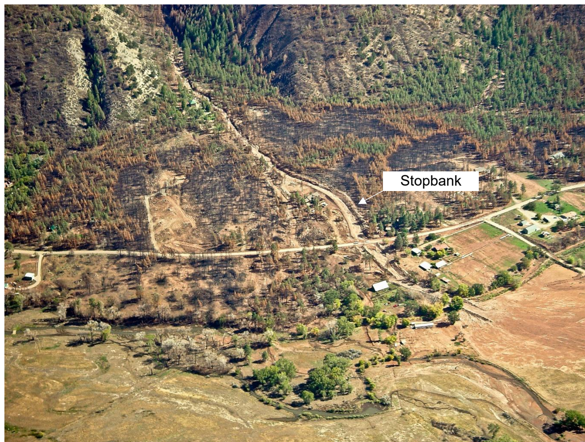
Figure 4: The Kroeger Canyon alluvial fan, Colorado with stopbanks following a fire in 2002 (Colorado Geological Survey, n.d.).
