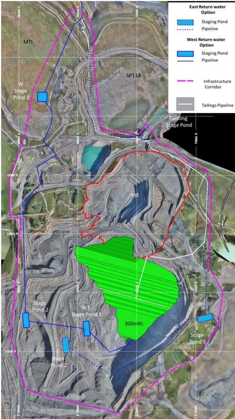
Figure 12.3 FTFS return water pumping system, showing staging ponds
