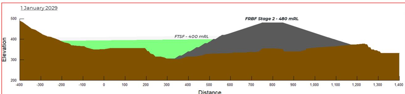
Figure 6.1 FRBF and FTSF filling level at the end of IMOP mining downstream
