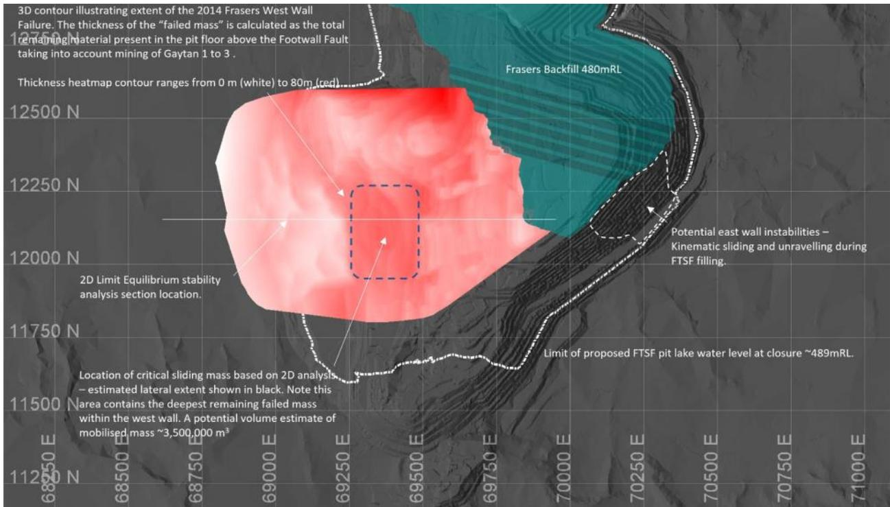
Figure 11.2 PFMs with increased susceptibility during FTFS operation (PSM 2024)
