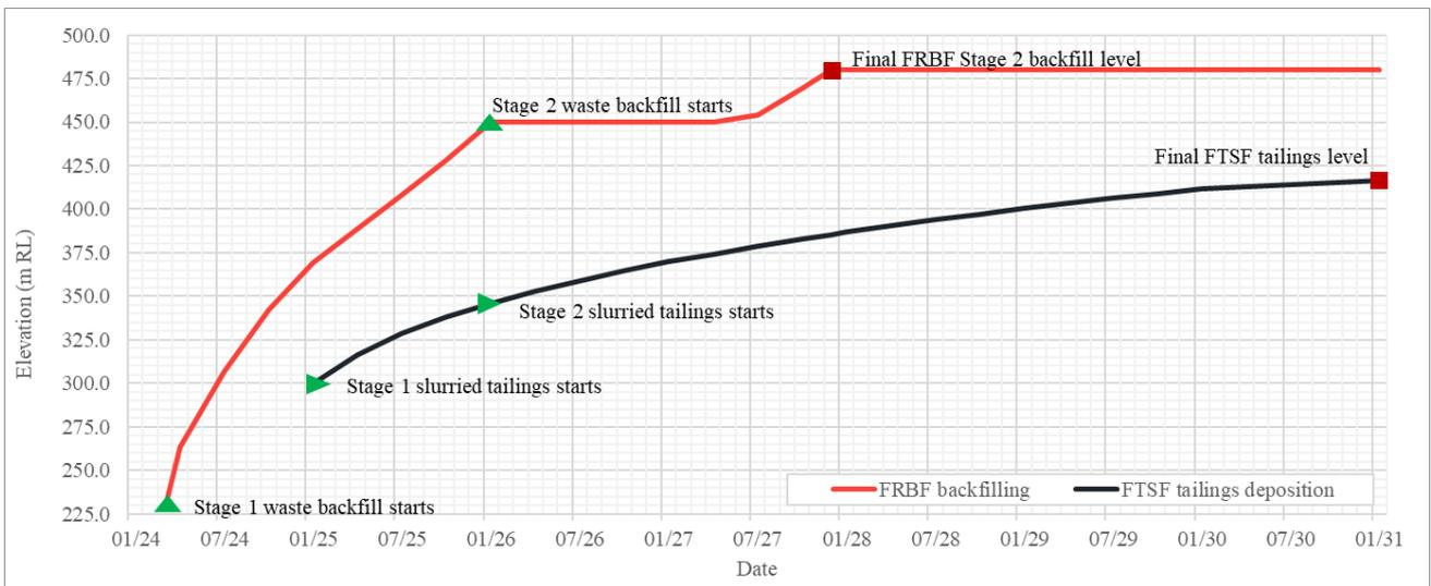
Figure 12.6 Projected FRBF tailings level and backfill crest during construction and operation
