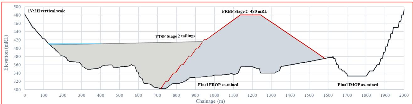
Figure 2.4 Cross-section through pits and FRBF, showing elevation of final FTSF tailings (1V:2H exaggeration)
