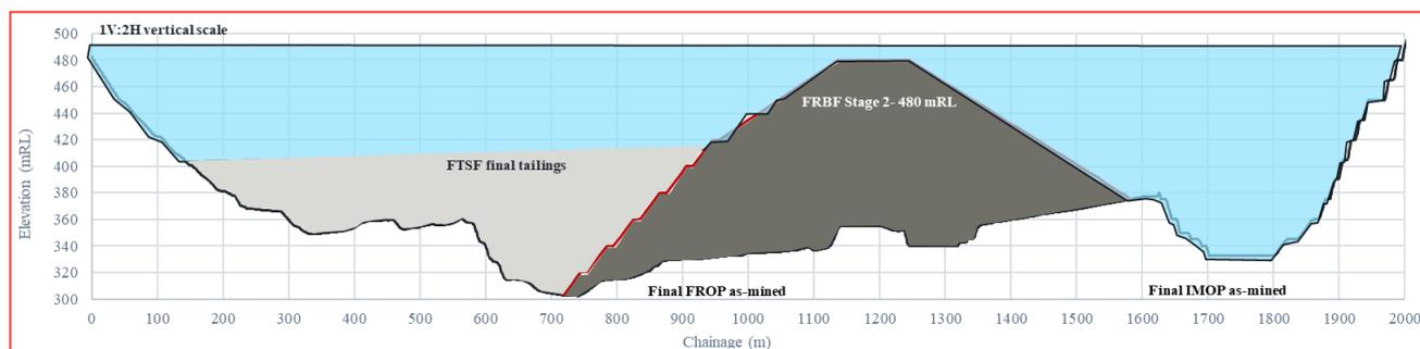
Figure 2.6 Cross-section through pits and FRBF, showing long-term pit lake elevation
