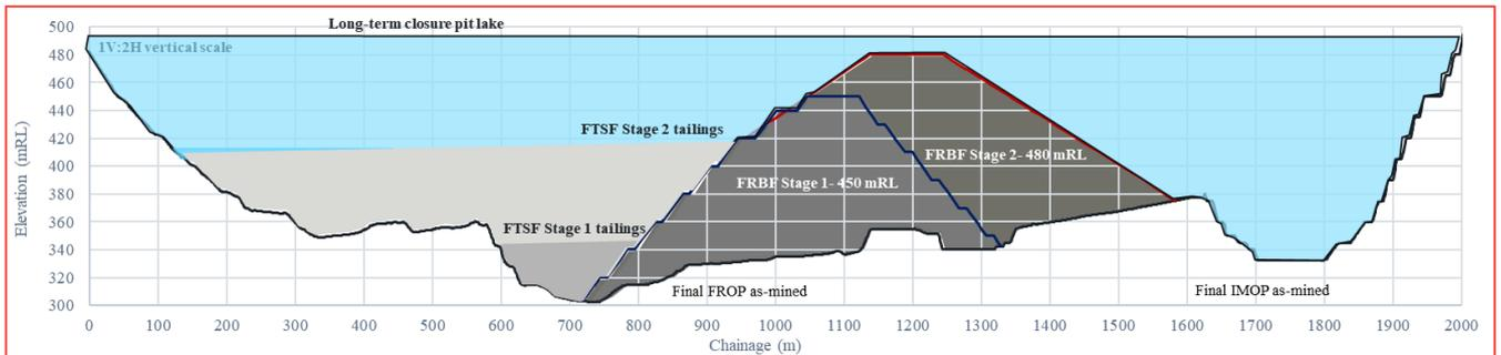
Figure 7.7 FTSF closure (stage 1 or Stage 2) pit lake cross-section
