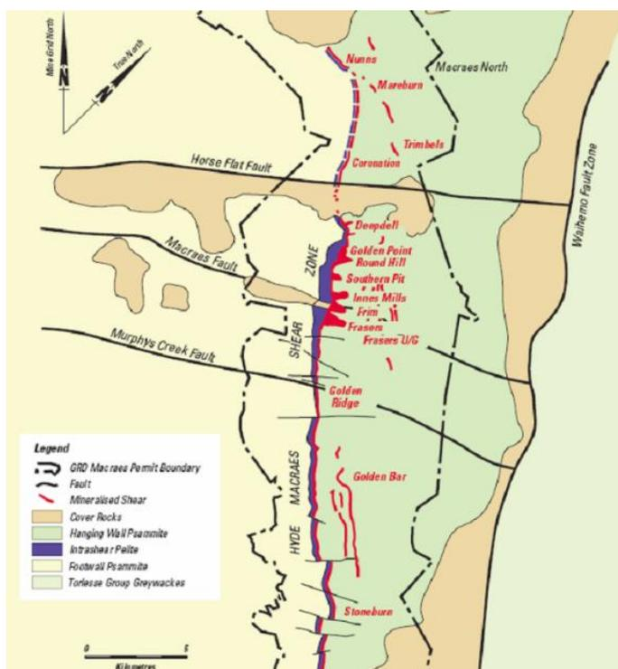
Figure 4.2 Plan of Macraes Mine showing various pits, deposits and the HMSZ (PSM 2022)
