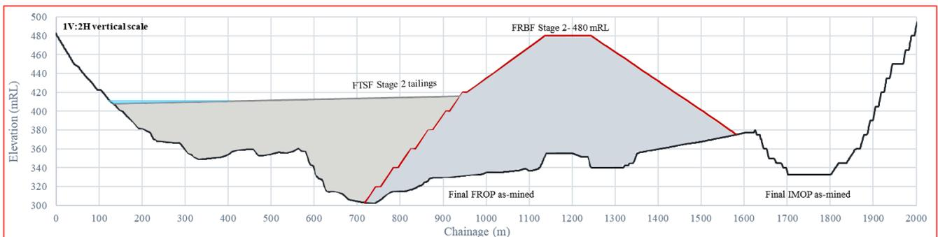
Figure 7.4 FTSF Stage 2 operational cross-section
