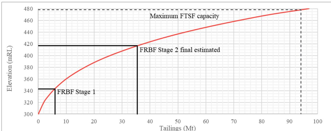
Figure 12.4 FTSF tailings stage-storage filling curve to FRBF crest
