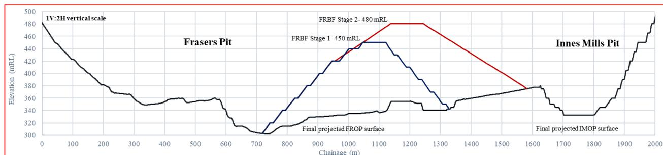
Figure 2.3 Cross-section through pits and FRBF, showing configuration of Stage 1 and 2 (1V:2H exaggeration)
