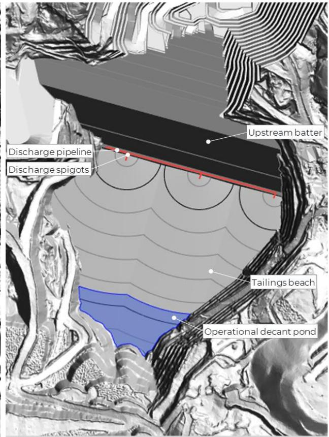
Figure 12.2 Plan of Stage 2 tailings operations (end of operations)
