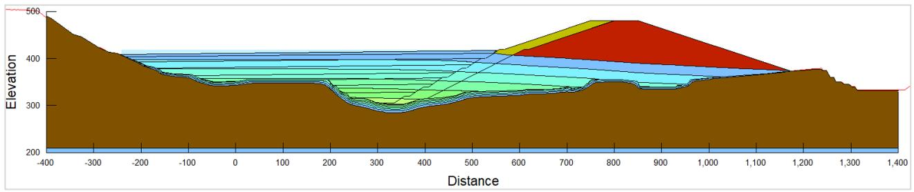
Figure 8.2 Phreatic surface through FRBF adopted for stability modelling at the end of FTSF Stage 2
