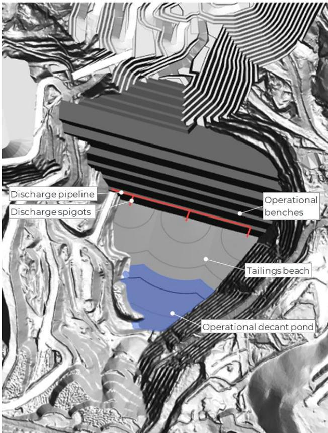
Figure 12.1 Plan of Stage 2 tailings operations (beginning)
