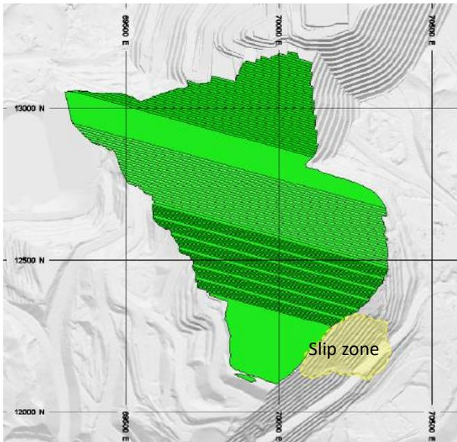
Figure 11.1 Slip zone in east high wall
