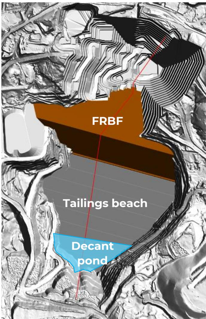
Figure 2.5 Plan of final tailings beaching against FRBF Stage 2
