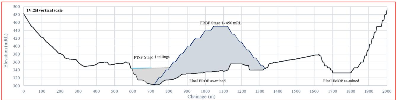
Figure 7.3 FTSF Stage 1 operational cross-section
