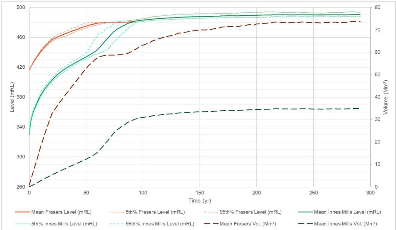
Figure 2.7 FTSF and IMOP pit water filling model over time
