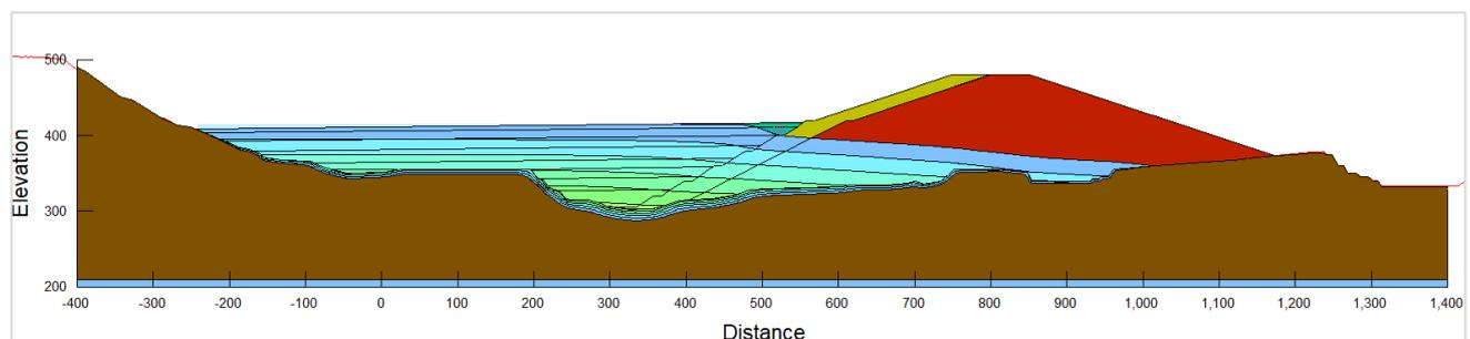
Figure 8.1 Seepage pathway modelled through FRBF at the end of FTSF Stage 2
