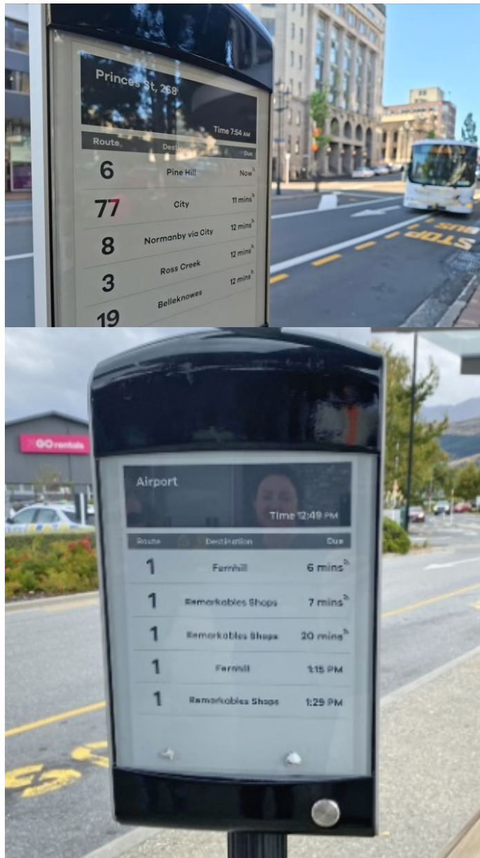
Figure 3: E-stop on Princes Street, Dunedin and Queenstown Airport
